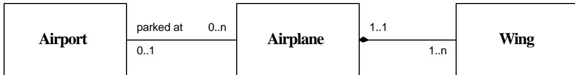
Figure 9. The difference between instance and aggregation relationships.
